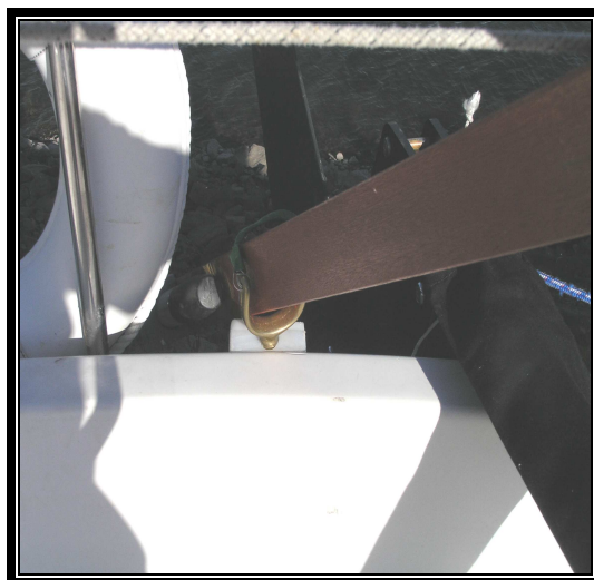
Emergency tiller to Starboard of regular tiller
