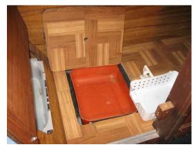
The area under the flip up portion of the settee was not useful. To port a drawer insert from Ikea was secured under the fixed portion of the settee. The cabin sole to port of the head was then opened up with an access hatch. Though the area under is only about 4" deep, by employing an assortment of modified plastic bins it is a great place to store a lot of drinking water bottles.
