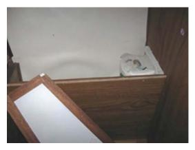
The area immediately behind the head was just a curved hull. By squaring it off and building a concealed lid a useful and secure storage space is created.
