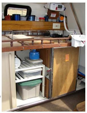
The space to the right of the icebox holds binoculars and our board mounted compass when not in use (In use, the board & compass fit in the companionway.) The stove is a replacement for the original Bluet and uses resealable Camping Gaz canisters.
