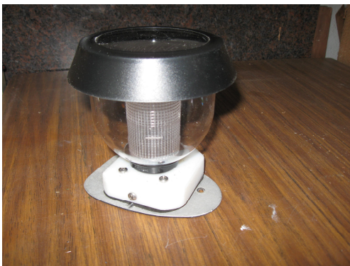
HDPE base attached to top plate of the mast.
