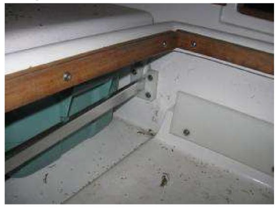
I slide the hatch in with the hinge towards the hull. I place a sponge between the halves which slightly opens the parts like a "relaxed" oyster. It slides under the seat and then opens slightly and catches on the lip so it will never come out. I've had the boat way over and it never came out. It frees space in the cabin and is easily accessible when I want to put the hatch back in place on short notice.
