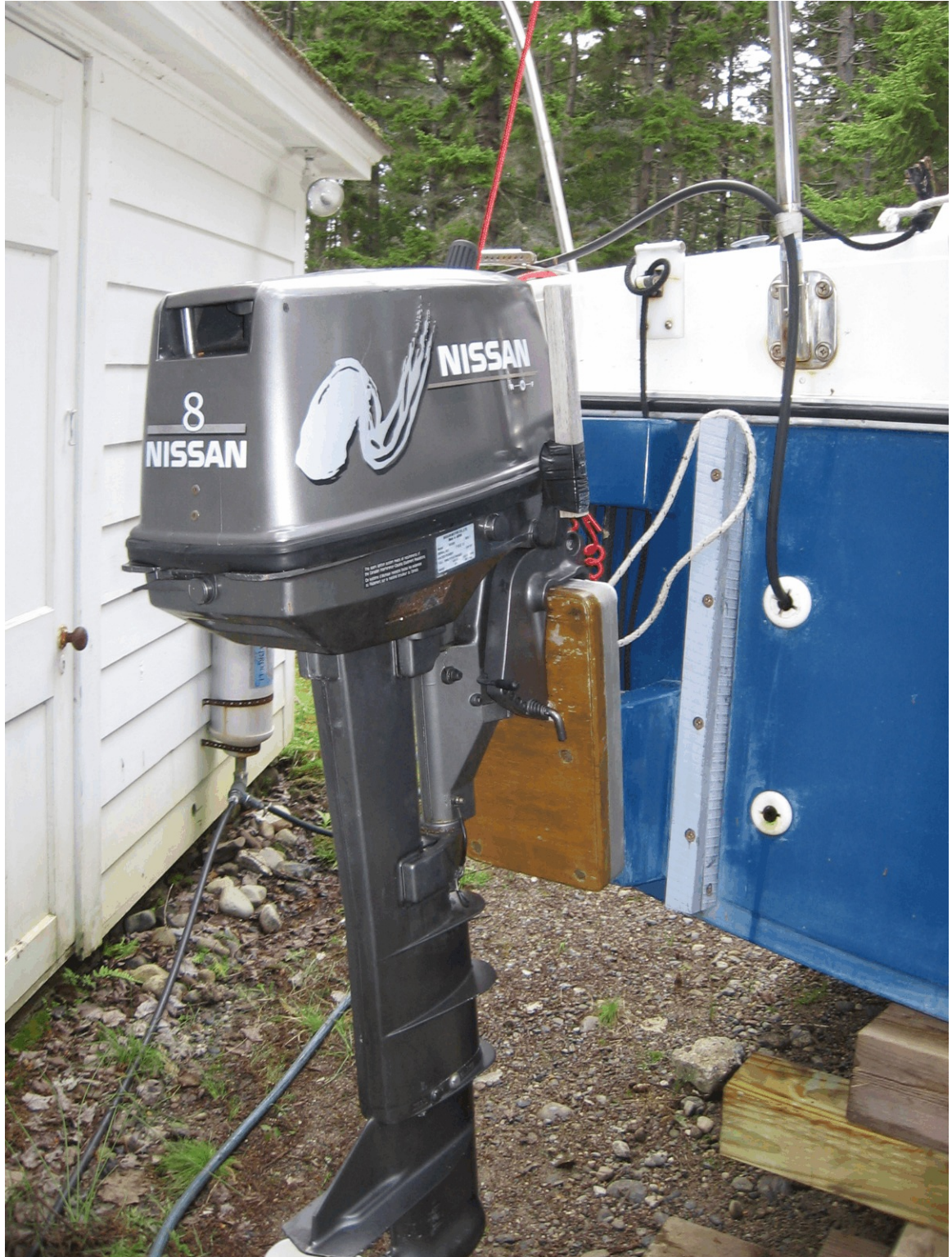
Nissan/Tohatsu 8 hp long shaft outboard. Weighs less than 60 lbs, usually starts on one pull, often with no choking required.
