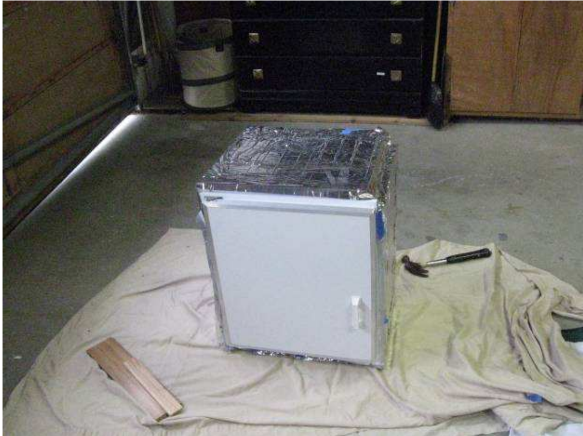
Completed box with Double Thick Panels on Bottom and Back
