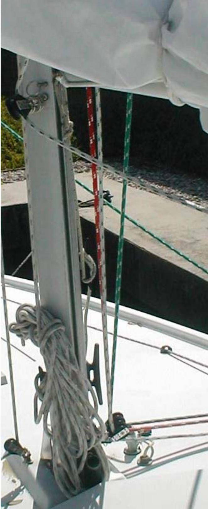
The (white with green spots) reefing line is lead thru the port mast block up through the reefing cringle on the port side and down through the triple
