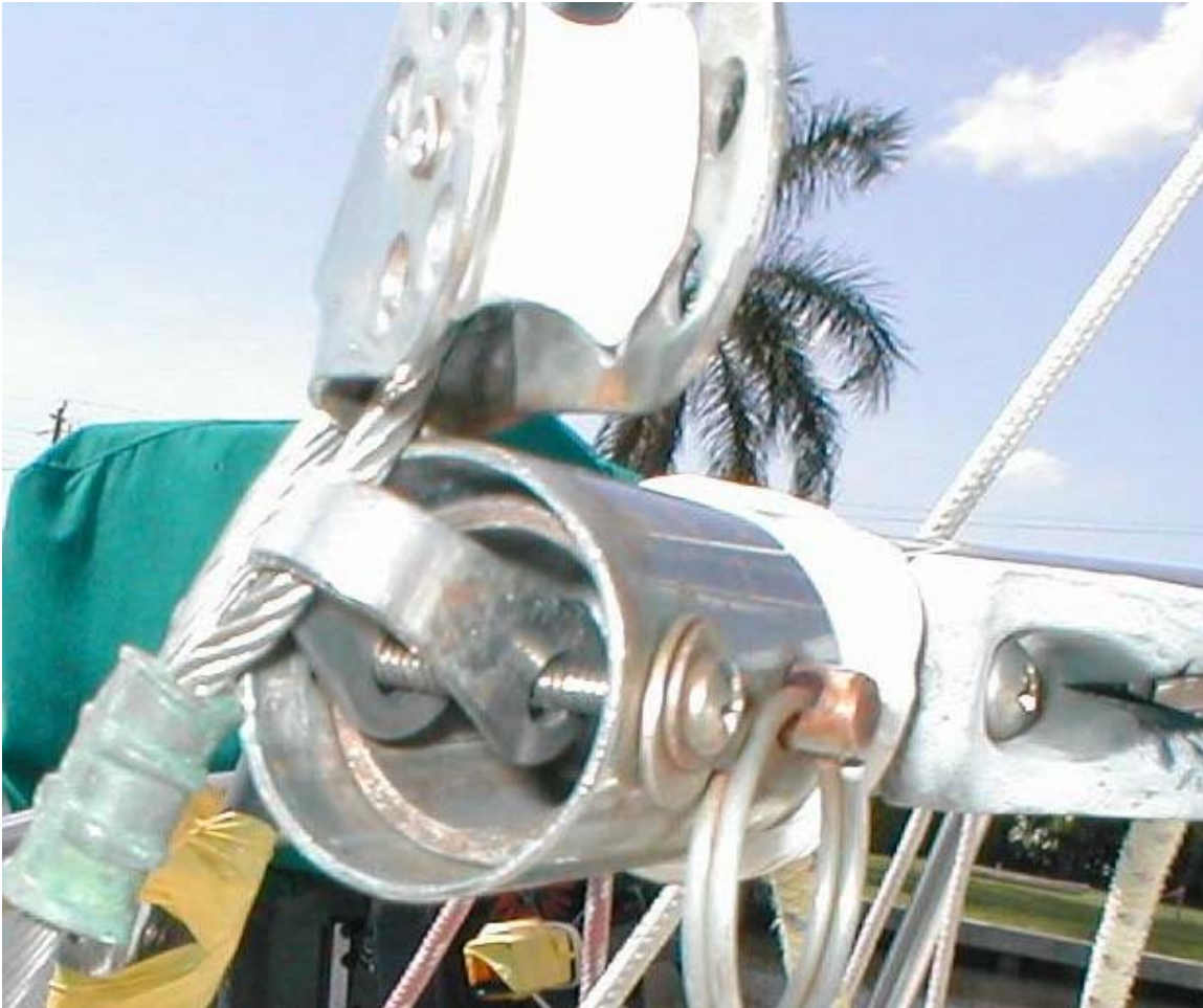
Detail of shackle, throughbolt, bar attachment fast-pin, and wire cable. You'll note that I haven't gotten around to cutting the old bullet blocks off.
