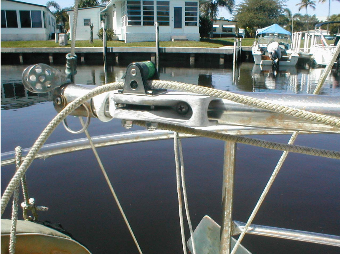
Starboard traveler cleat throughbolted to clam cleat. Note the old blocks for the older type traveler.
