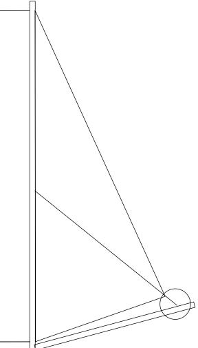
The clew outhaul rides on an adjustable car. To power up adjust the fore and aft position so the clew outhaul control line, extended straight, intersects the mid point of the luff. Or, to open up the top of the leech, move it aft.
